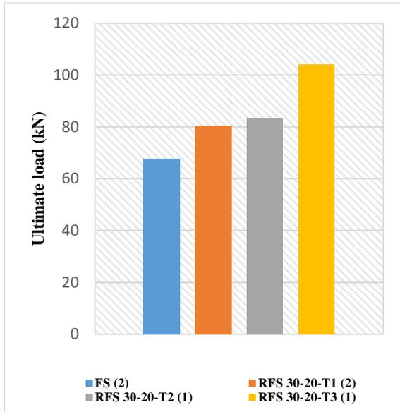
**Fig 7: Comparison chart for 20mm CFRP strips specimens with FS (2)**
