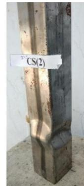
**Fig 3: failure modes of CS (2)**
