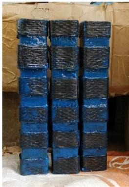
**Fig 2: Fire exposed specimens wrapped with 20mm of CFRP strips**
