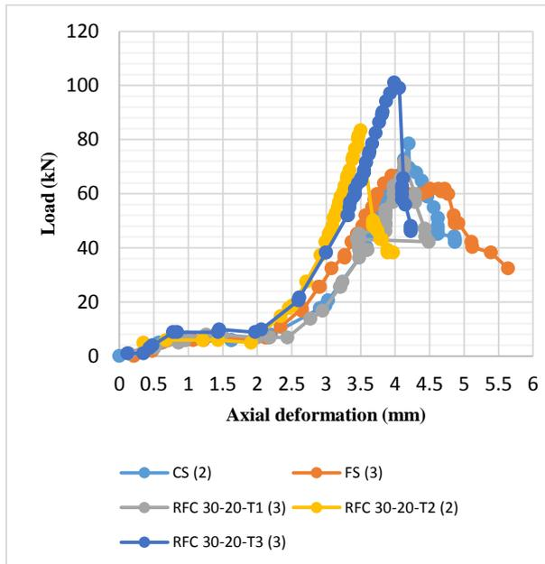
Fig 6: Comparison of axial load-deformation behaviour
